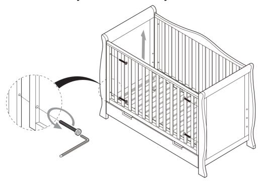
Loose the four screws of 4PCS M6X55mm bolt(c) by Allen Key(d) as above photo and the sofa will be ready as below.
