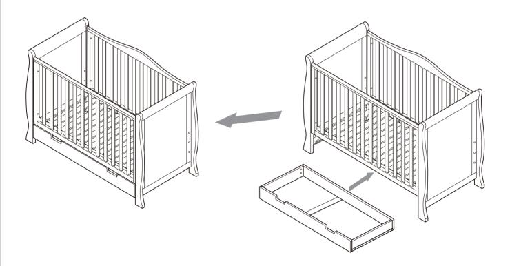
Slide assembled drawer into the runner on the cot ends.
