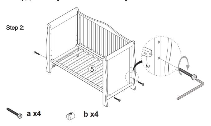
Connect base(5)to the left end (1) and right end(2) with 4PCS M6 X70mm bolt (a) by Allen Key (d).
