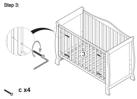
Connect the other fixed side (3) to left end(1) and right end (2) with 4PCS M6X55 bolt(c) by Allen Key(d)Tighten all the bolts.
