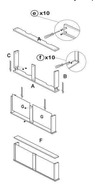
**Step1:** Insert 6PCS(e) Metal Pin to (A) front panel as diagram.
